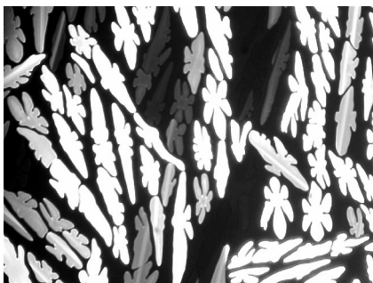
FIG. 1. Typical polarizing microscopic texture of the liquid crystalline “banana” B1 phase, showing clear features of dendritic growth. The image size is 520 \mu\text{m} \times 390 \mu\text{m} .
